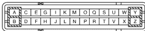
ABS HU/CM WIRING HARNESS-SIDE CONNECTOR
